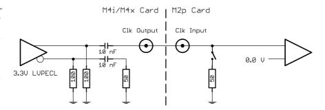
Due to the programmable threshold level of the M2p card, the M4i/M4x clock output can be directly connected to the M2p DC-coupled clock input, when setting the threshhold to zero Volt.
