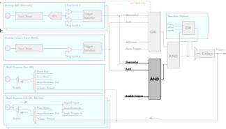
Every trigger source of the M2p series cards except the software trigger is wired to one of the above mentioned AND masks. The user then can program which trigger source will be recognized, and which one won't.
