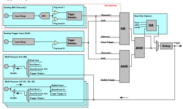
The trigger engine of the M2p card series allows to combine several different trigger sources with OR and AND combination, with a trigger delay or even with an OR combination across several cards when using the Star-Hub option. The above drawing gives a complete overview of the trigger engine and shows all possible features that are available.
