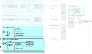
The multi purpose I/O lines are available on the front plate and labeled with XO (line 0), X1 (line 1), X2 (line 2) and X3 (line 3). As default these lines are switched off.
