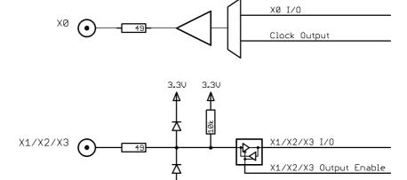
series resistor for logic levels up to 5.0V. To avoid floating levels with unconnected inputs, a pull up resistor of 10 kOhm to 3.3V is used on each line.
