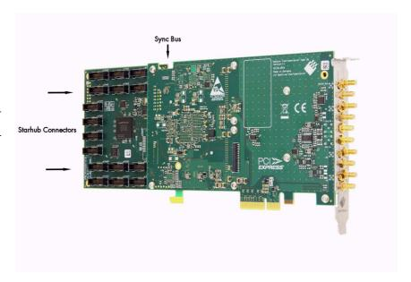
The module acts as a star hub for clock and trigger signals. Each board is connected with a small cable of the same length, even the master board. That minimizes the clock skew between the different cards. The picture shows the extension module mounted on the base board schematically without any cables to achieve a better visibility.
