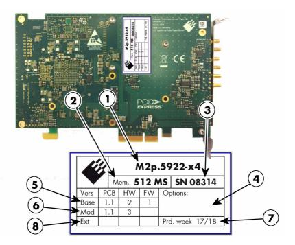
The Spectrum type plate, which consists of the following components, can be found on all of our boards. Please check whether the printed information is the same as the information on your delivery note. All this information can also be read out by software:
