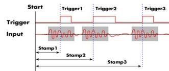
The timestamp function writes the time positions of the trigger events in an extra memory. The timestamps are relative to the start of recording, a defined zero time, ex-
