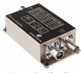
For the acquisition of extremely small voltage levels with a high bandwidth a series of external amplifiers is available. Each of the one channel amplifiers is working with a fixed input impedance and allowsdepending on the bandwidth to select different amplification levels between x10 (20 dB) up to x1000 (60 dB). Us-
